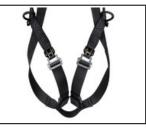
The leg loops are equipped with FAST LT automatic buckles, allowing the harness to be easily donned with both feet on the ground. These buckles retain their adjustment settings between donnings.
